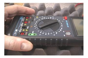
Finish tightening the case screws. CAUTION! Don't over tighten metal screws into a plastic case or you may permanently damage your meter.
