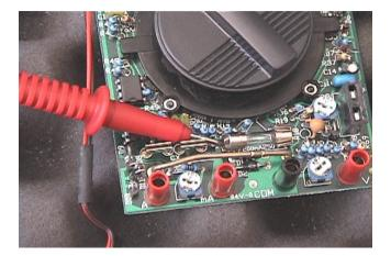
If you look through the new fuse into a light source, you may be able to see the tiny wire. Locate the new fuse on the fuse holder prongs. Press down with equal force across the entire fuse.
