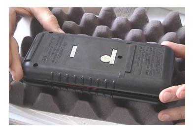
Start the 3 identical case screws by hand. If you encounter resistance, reverse the screw direction until there is no resistance and start again. The screws are going into plastic. You do not want to cut new threads. Instead you want to feel the screw threads following the old threads.
