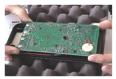
When the board is in place, the level of the board will match the level of the battery holder. You may also turn the meter over to check for jack and switch alignment.
