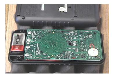
Carefully lift the battery and connector out of the battery compartment. Notice the routing of the battery cable through the case slot. Remove the battery.
