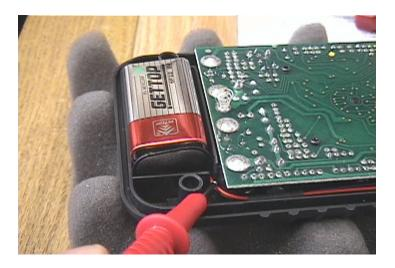
Using both hands, gently guide the back case over the circuit board. Do not force.
