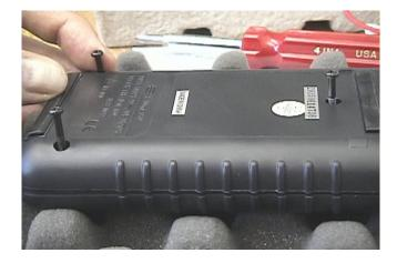
Start tightening each of the 3 screws, in a 1-2-3-1-2-3 sequence, to make sure all screws are seating correctly and the required force is small. If a screw seems tight, reverse directions, to avoid cutting new threads, and start over.
