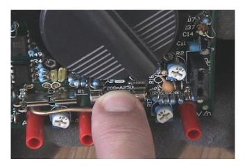
Using both hands, gently guide the board back into the case. Be careful not to force the board or bend any components.
