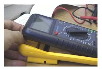
Turn the meter on its face on a soft surface. Unscrew the 3 identical screws with a #2 Phillips screwdriver. The screws have a right-hand thread, so turn the screwdriver counter-clockwise. CAUTION! Using a screwdriver that is too small or too large may permanently damage the meter case screws. It is not necessary to remove the screws, but you may have less difficulty with the next step if you do.
