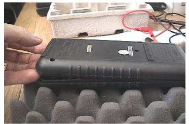
Guide the case back straight up from the meter, being careful not to bend any internal parts.
