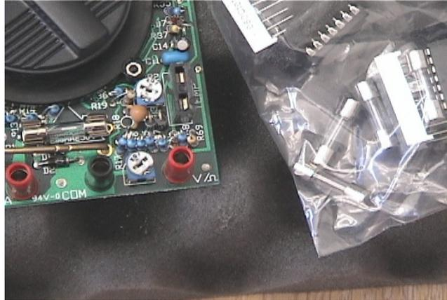
Turn the circuit board over on the soft surface. Find the 200 mA fuse. Note the thick wire with the crimps in it. This is the precision current shunt, which should be protected. Use a meter probe to gently pry one side of the fuse out of its holder. Lift out the old fuse with your fingers.
