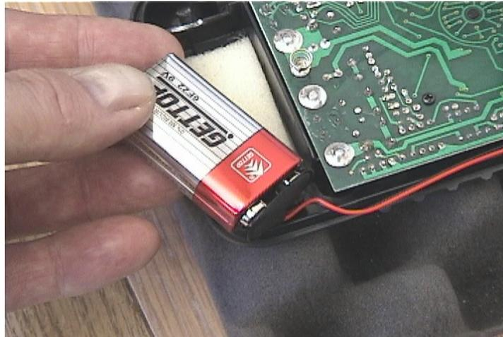
Using a meter probe, guide the battery wires into the case slot. Note the relative location of the black insulation on the battery wires.
