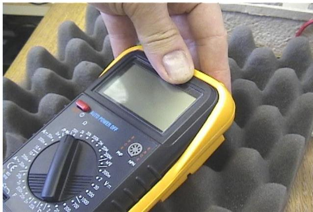
Perform a simple ohms test to make sure your meter is operating.
