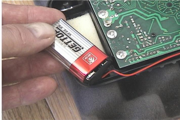
Lift the circuit board straight up, using both hands. Continue working on a soft surface.
