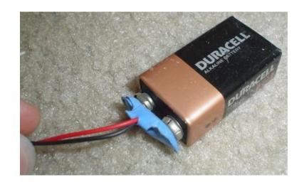
7. Use a meter probe to guide the battery wires into the case slot. Note the relative location of the black insulation on the battery wires.
