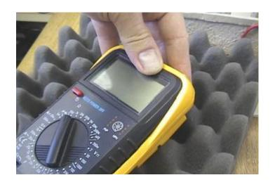
13. Perform a simple ohms test to make sure your meter is operating. You should have an overflow with the leads separated, and close to  $0\Omega$  with the leads shorted together.
