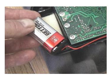
6. Install the 9 volt battery, aligning the battery terminals correctly to the battery connector. Press the connector firmly onto the battery.
