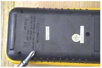
CAUTION! Using the wrong size screwdriver may permanently damage the screws. It is not necessary to remove the screws from the cover, but you may have less difficulty with the next step if you do.
