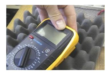
13. Perform a simple ohms test to make sure your meter is operating. You should have an overflow with the leads separated, and close to  $0\Omega$  with the leads shorted together.
